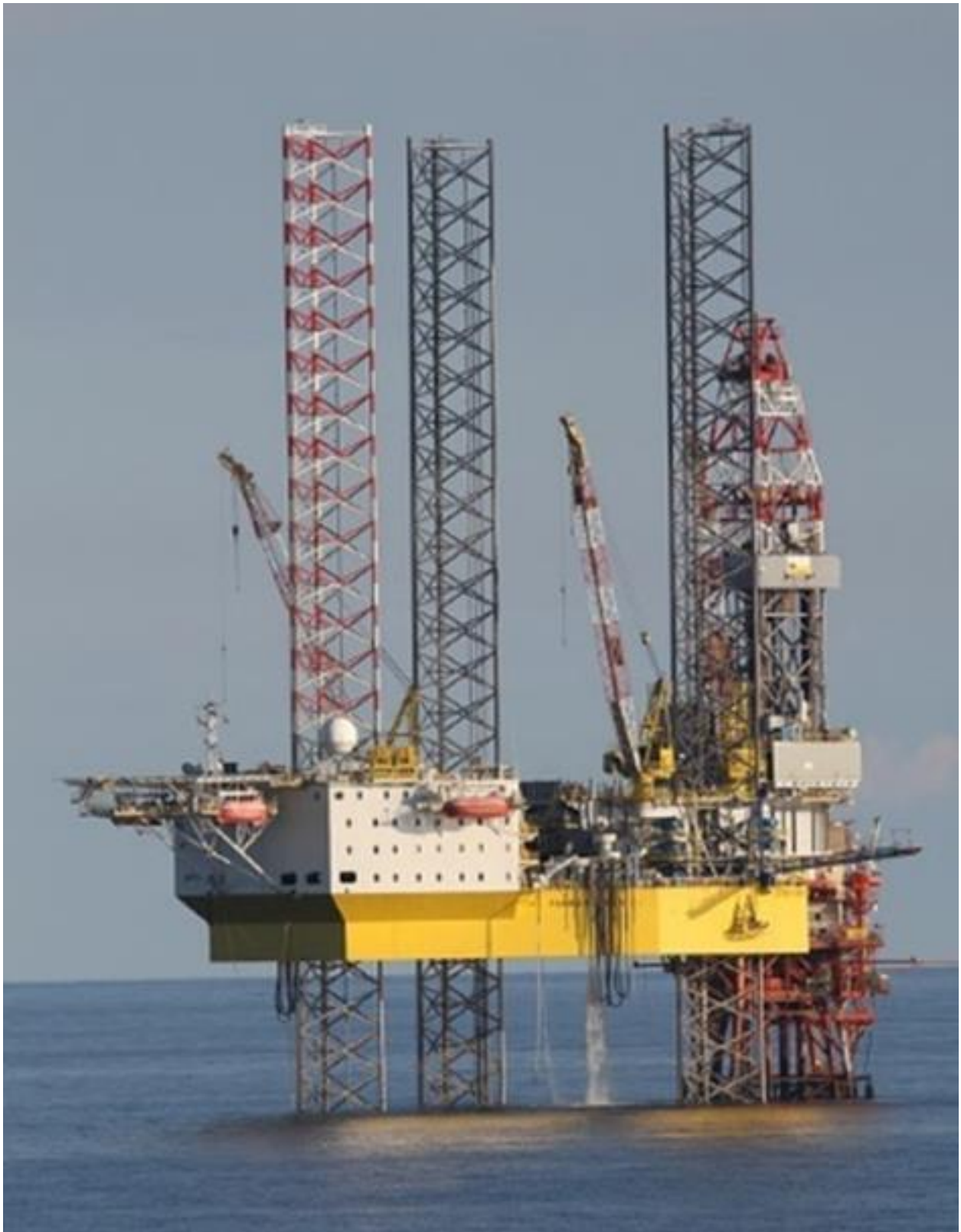
This shallow-water jack-up, drilling in water depths of 200m or less, will cost between $30k and $50k per day. Courtesy of Pixabay
